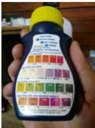
Simple water testing equipment that can measure pH, turbidity and residual chlorine
